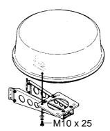
(B) Fastening antenna to mounting bracket
